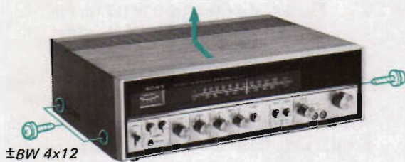
Fig. 2-1. Wooden case removal
