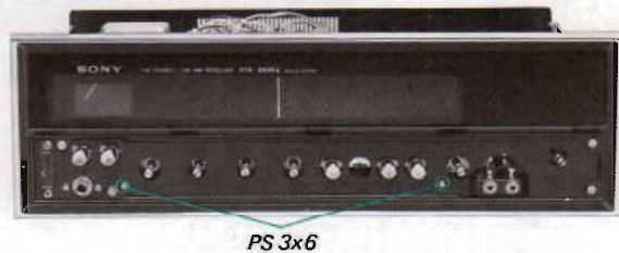
Fig. 2-12. Control circuit board removal
